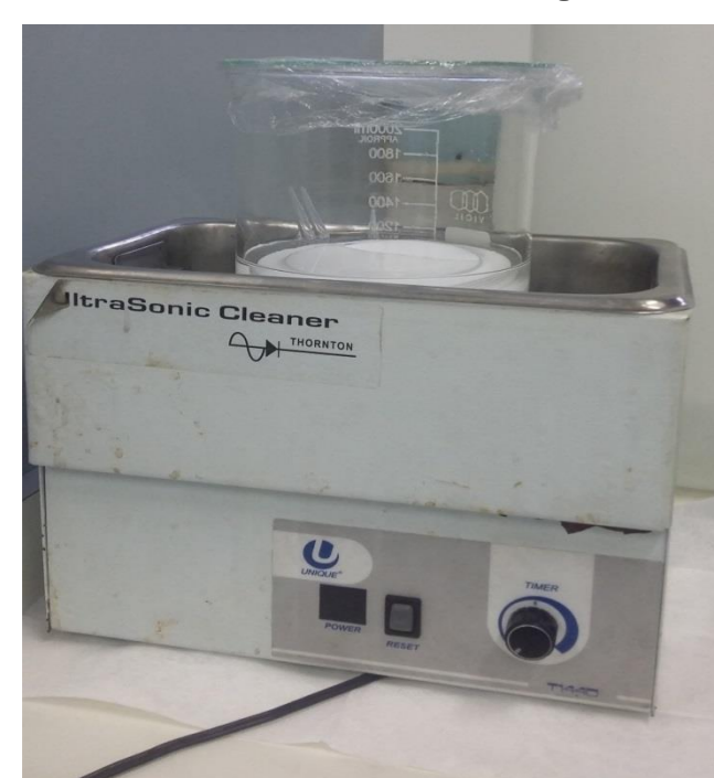
Fig.4 - Tubes and pipette tips sonicated with 50% (v/v) HNO 3 solution 30 minutes before being used.
