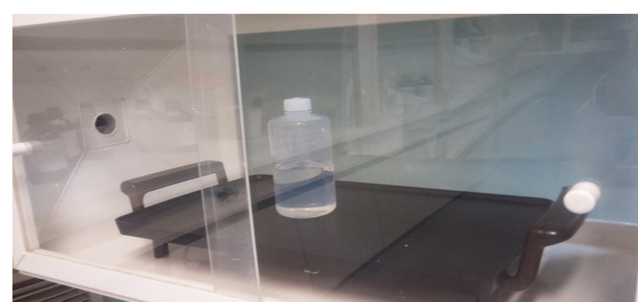
Fig.5 - Bottles are half filled with the 50% (v/v) HNO 3 solution and heated at 60 °C for a week.
