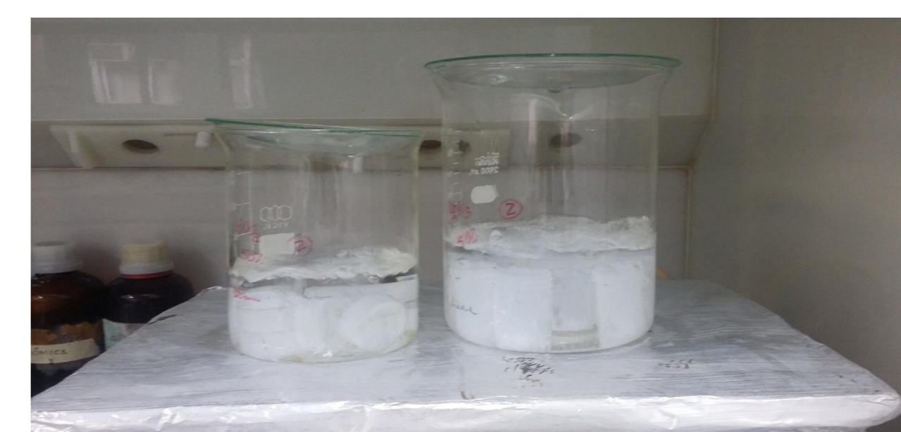
Fig.6 - Savillex® teflon beakers boiling in 50% (v/v) HNO 3 .
