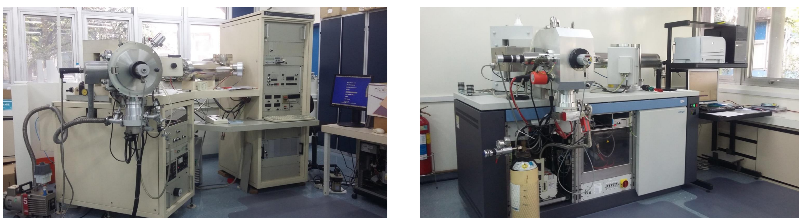
Figure 2 – Mass spectrometers at CPGeo: A- Finnigan MAT 262; B- Thermo Triton
